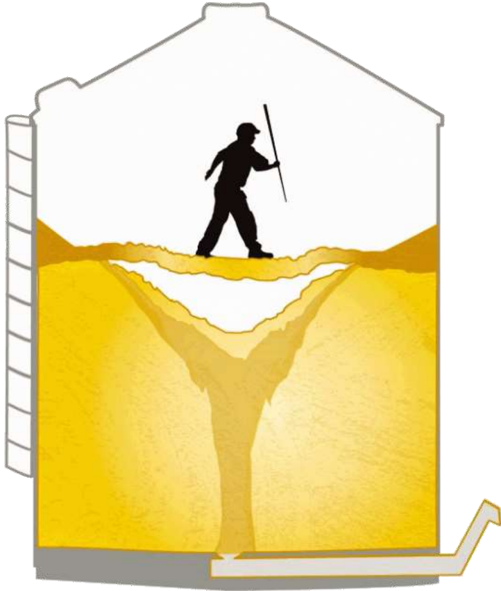
Crust forms on top Void created when bin is emptied
