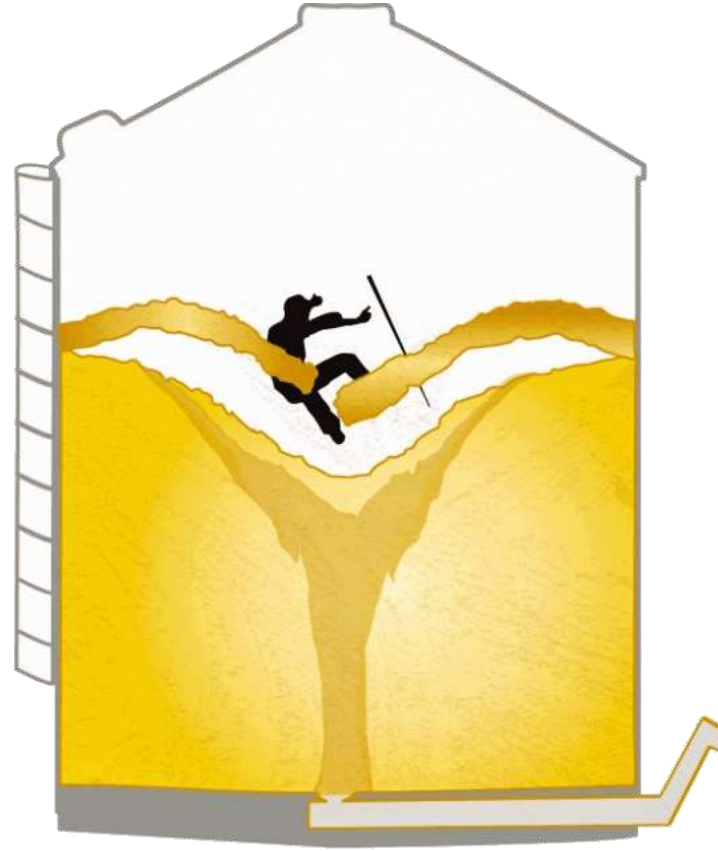
Collapse when walked on
